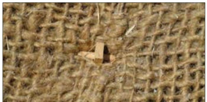
Figure 5: Jute net with wooden pin
